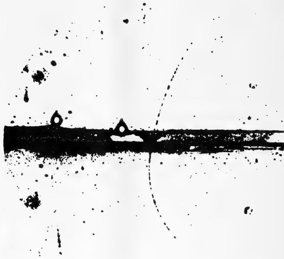
Fig. 12.—Photograph of a ray losing energy in a lead plate. A greater curvature of the track in the lower half of the photograph is noted corresponding to a lower energy after it has emerged from the lead. (From Anderson.)
